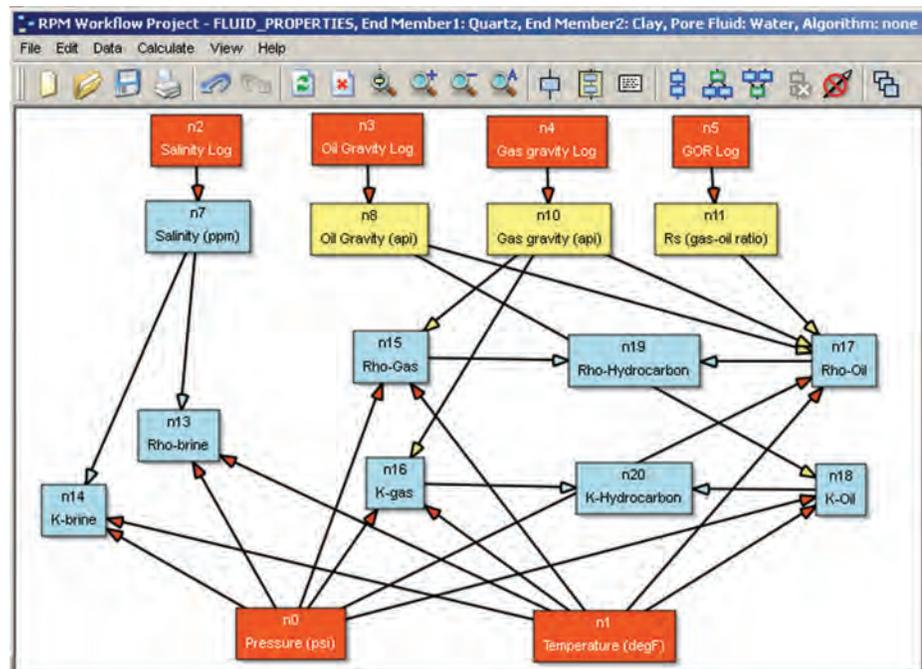
Figure 5: PowerLog with RPM features graphical workflow. Each node shown here represents inputs or calculations, with arrows indicating the flow between nodes. Node sets can be grouped into functions through color-coding. Workflows can be saved and applied to new log sets.
