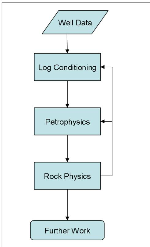
Figure 2: Some people consider integration of rock physics with petrophysics to be achieved when both analyses are included in the workflow. However, the model, processes, and parameters are not consistent and iteration is difficult because the well files typically have to be moved between applications.
