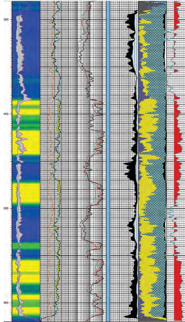
Figure 1: Petrophysics combines well log, core, mudlog, and other disparate data sources for the purpose of evaluating, predicting, and establishing formation lithology.
