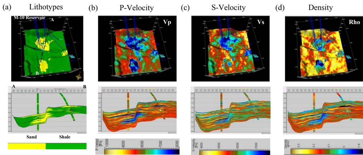
Figure 3. AVA stochastic inversion results: (a) Lithotypes (sand/shale); (b) P-Velocity; (c) S-Velocity; and (d) Density. The spatial coverage is approximately 4 km<sup>2</sup>, and the vertical interval: 3500-4300 ms.
