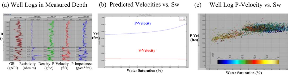
Figure 1. (a) Fluid/lithology sensitivity well logs showing the characteristic low values of P-velocity, density, and acoustic impedance for hydrocarbon-bearing sands; (b) Cross-plot of predicted P- and S-velocities vs. water saturation using Biot-Gassmann equations: P-velocity clearly decreases when hydrocarbon saturation increases. This behavior is also indicated by well log data (Panel c).
