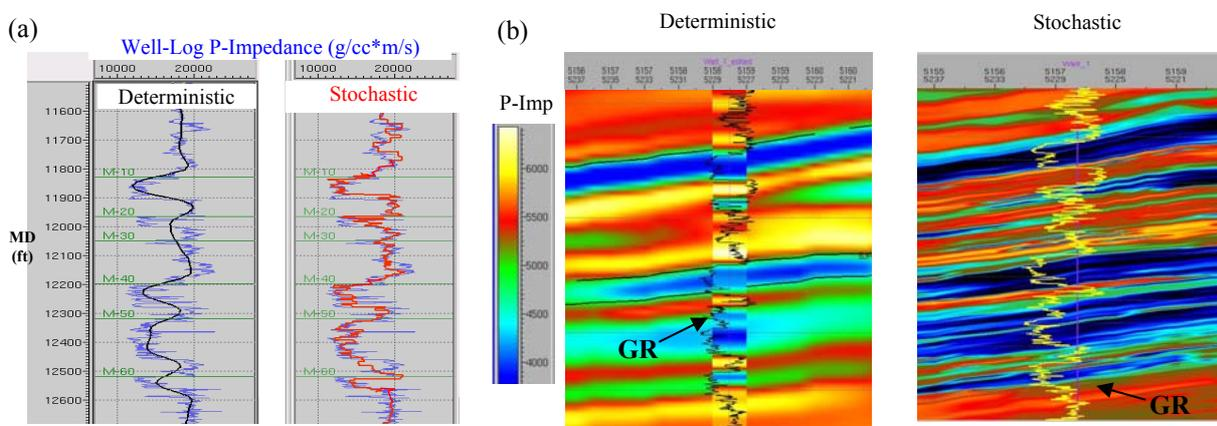
Figure 4. Deterministic versus stochastic inversion results: (a) inverted P-impedance pseudo logs extracted at a well location; (b) inverted P-impedance cross-sections. Deterministic results are sampled at 4 ms whereas stochastic inversion results are sampled at 1 ms. Vertical interval: 3800-4300 ms.
