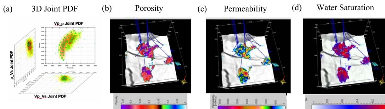
Figure 5. (a) 3D joint PDF of acoustic properties (six properties were used for co-simulation: P-Velocity, S-Velocity, density, porosity, permeability, and water saturation). (b), (c), and (d) Co-simulated porosity, permeability, and water saturation, respectively, for the M-10 reservoir.
