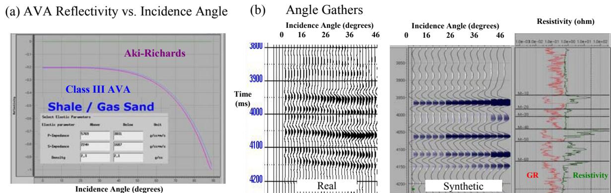
Figure 2. AVA sensitivity analysis results: (a) AVA reflectivity at the shale/gas-sand (M-10) interface, showing a Class III AVA response; (b) comparison between real angle gathers (left) and synthetic angle gathers (right) generated from well-log data indicate an increase in amplitude with an increase of the angle of incidence.
