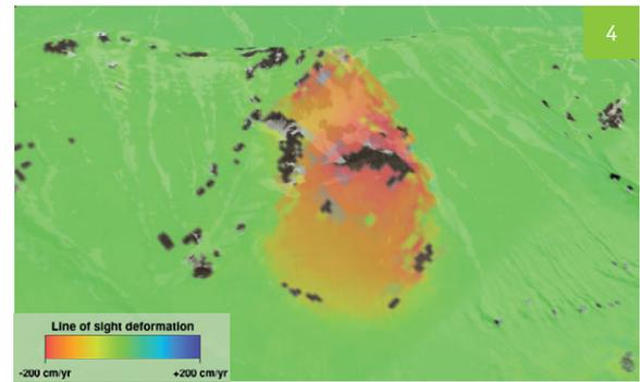
Figure 4. Oblique view of the cumulative displacement associated with the Fagraskógarfjall landslide, spanning July to November 2017. The upper and middle portions of the landslide were moving significantly faster than the lower portion. The area of greatest movement is associated with a steeper area of the hillside. Measurement gaps along the landslide primarily relate to rapid levels of deformation © CGG 2018. Images contain modified Copernicus Sentinel data (2018).
