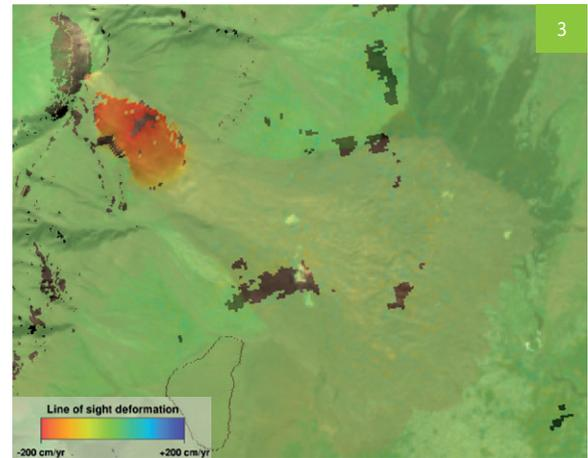
Figure 3. Yearly rate map of the Fagraskógarfjall landslide between July and November 2017. Green represents relatively stable areas while the red-yellow region highlights significant slip of the landslide. Up to 2 m per year of slip may have occurred in some parts of the landslide. © CGG 2018. Images contain modified Copernicus Sentinel data (2018).
