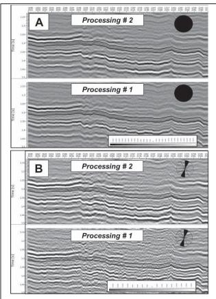
Figure 2: A - Comparison of seismic sections obtained with different processing flows : A) full stack, full azimuth sections; B) partial stacks in a azimuth sector
