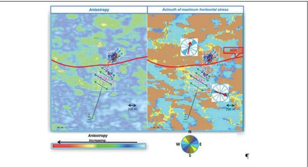
Figure 6: Comparison of the predicted azimuth of the maximum horizontal stress and the azimuth of the hydraulic fractures from microseismic.
