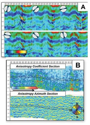
Figure 1: Figure 1. Pre-stack azimuthal inversion results (A - Vp/Vs ratio for different azimuthal sectors; B –Anisotropy coefficient and maximum anisotropy azimuth sections).
