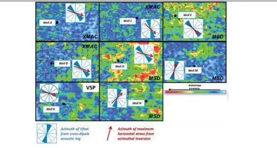
Figure 5: Comparison of the predicted azimuth of the maximum horizontal stress and of the azimuth of Vfast from crossdipole acoustic logs and a walkaway VSP at one well location.
