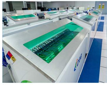
GPU nodes in oil cooling
