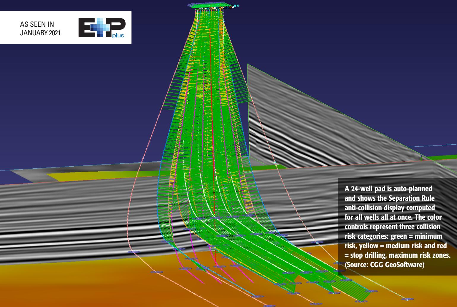
A 24-well pad is auto-planned and shows the Separation Rule anti-collision display computed for all wells all at once. The color controls represent three collision risk categories: green = minimum risk, yellow = medium risk and red = stop drilling, maximum risk zones. (Source: CGG GeoSoftware)
