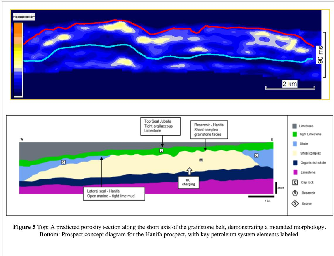
**Figure 5** Top: A predicted porosity section along the short axis of the grainstone belt, demonstrating a mounded morphology. Bottom: Prospect concept diagram for the Hanifa prospect, with key petroleum system elements labeled.
