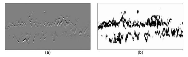
*Figure 3*: (a) Seismic responses of injectites predicted by applying our U-Net to Figure 1a; (d) Binary mask derived from (a).
