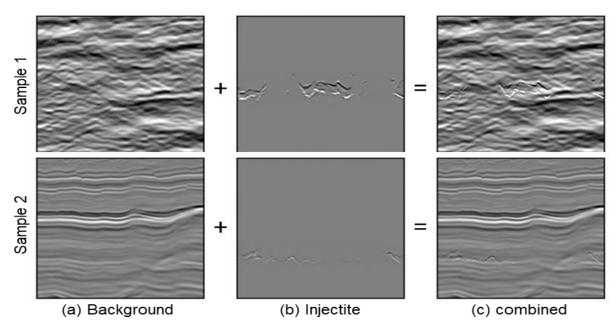
*Figure 2*: (a) Injectite-free seismic image as the background; (b) Seismic image of injectites from manual interpretation; (c) combined seismic image of (a) and (b)
