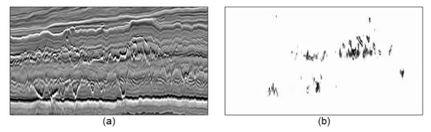
*Figure 1*: (a) Migrated seismic image that contains injectites; (b) Binary mask of injectites predicted by a conventional U-Net method.
