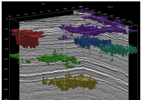
Figure 5: 3D visualization of injectite masks
