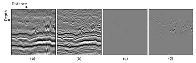
*Figure 6*: (a) Vintage seismic; (b) More recent seismic; (c) Model prediction from (a); (b) Model prediction from (b).
