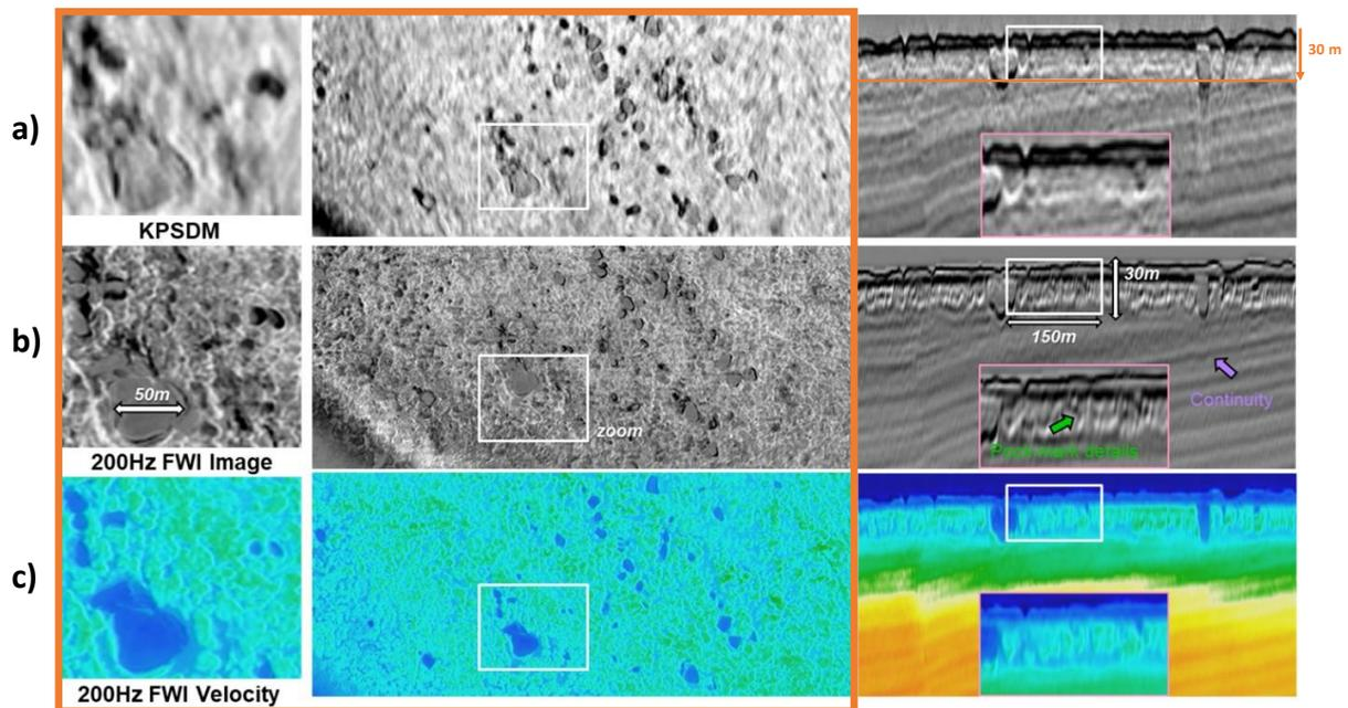
**Figure 4:** Shallow imaging uplift obtained with 200 Hz FWI; a) K-PSDM result, b) 200 Hz FWI Image and c) corresponding 200 Hz FWI velocity model.
