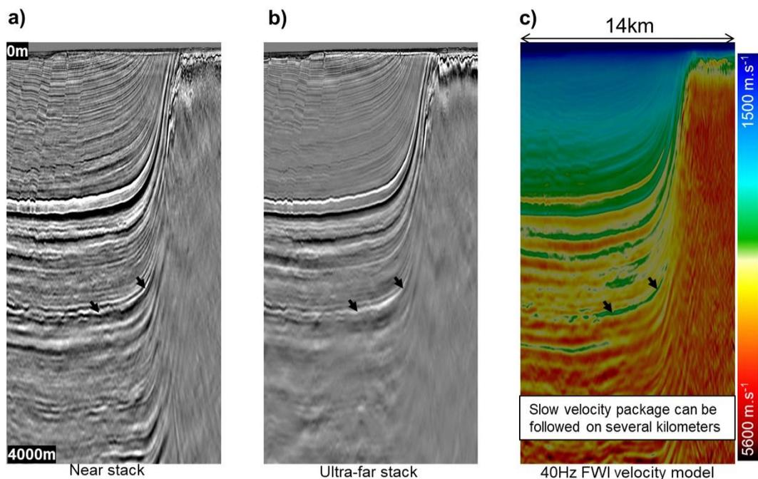
**Figure 3:** 40 Hz FWI: reverse-time migration (RTM) results for a) near stack and b) ultra-far stack. c) 40 Hz FWI velocity model used as final migration model.
