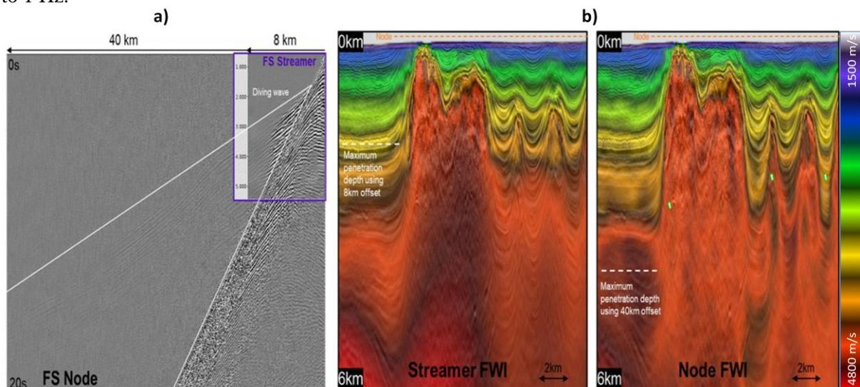
**Figure 2:** Uplift from node FWI over streamer FWI: a) Nordkapp ultra-long offset OBN gather after deblending; b) Comparison of streamer and node FWI – migrated seismic overlaid with velocity models; Orange dotted line shows the extent of the node carpet, deployed to cover the salt diapir area.
