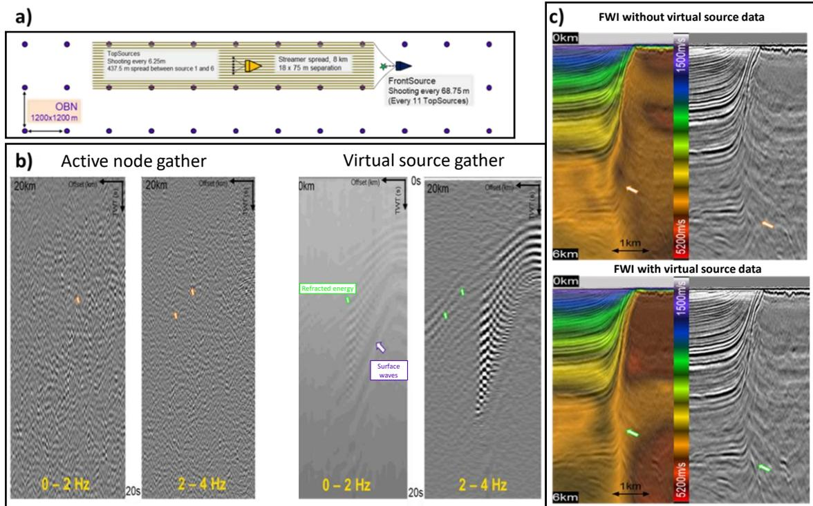
**Figure 1:** Node Interferometry; a) Hybrid acquisition design; b) Comparison of active seismic and virtual source gathers; c) FWI with and without interferometry gather contribution.
