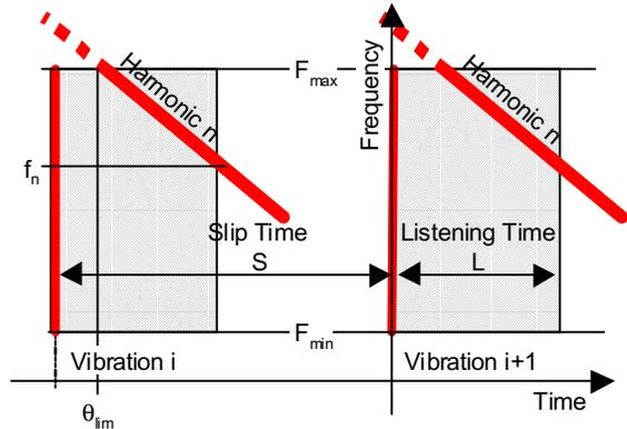
In slip-sweep operations, the interval between 2 consecutive sweeps, the slip-time, is too short to prevent interference between the harmonic noise and the previous record (see fig. 1). This interference can be described mathematically (P. Ras et al. 1999) as follows:
