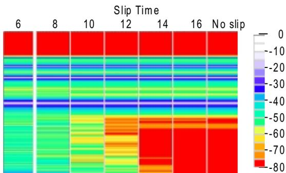
Fig.3 Variation in harmonic noise with slip time: The signal is an [8-80] 12s-linear sweep with 20% of H2 and H3, 12% of H4, 10% of H5 and 5% of H6. Data are NMO corrected and stacked (fold 60). Harmonic noise is found after the last reflection in blue.
