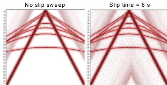
Fig.2 Comparison of conventional and slip-sweep data. In this example, radial noise is the major source of harmonic noise.
