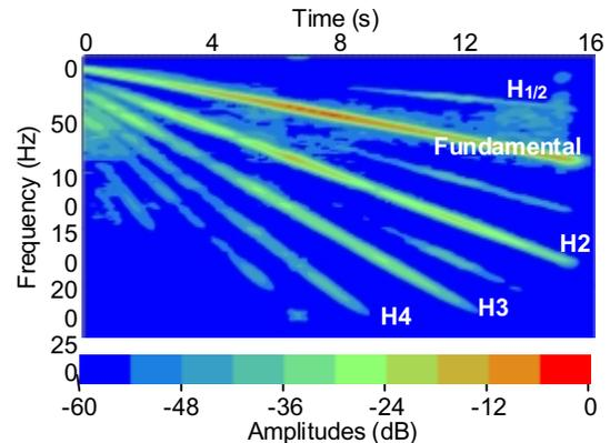
Fig. 4 Time frequency map of uncorrelated data. Note the relative strength of harmonics and sub-harmonics: the second harmonic rises from  $-24$  dB at 30 Hz up to  $-12$  dB at 80 Hz, the third harmonic is more consistent at  $-24$  dB. The 4<sup>th</sup> and 5<sup>th</sup> as well as the sub-harmonics remain below  $-30$  dB.
