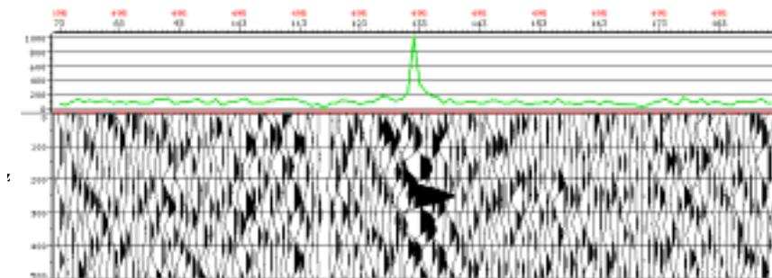
Figure 2 – Single hydrophone cross-correlations in the solid streamer
