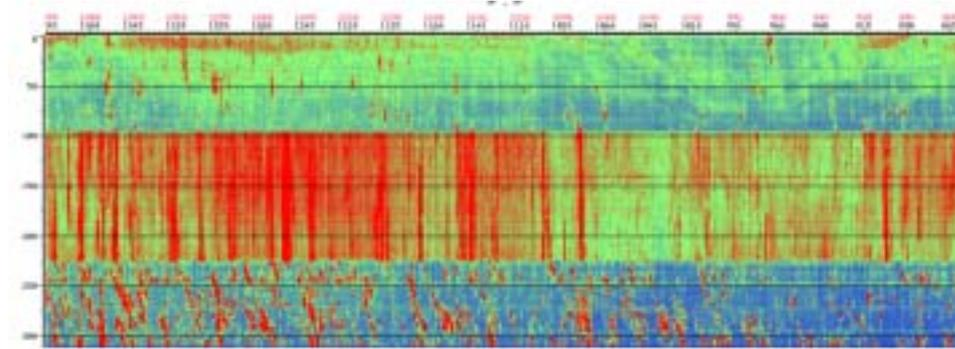
Figure 3 – RMS noise in solid groups, solid single hydrophones and liquid groups
