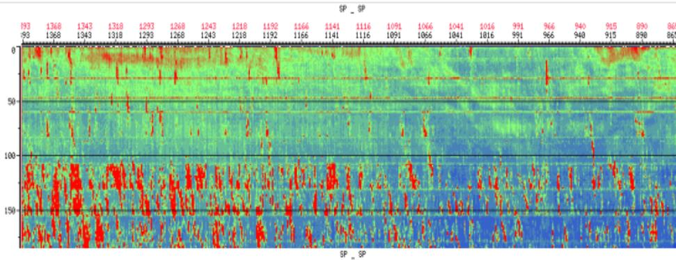
Figure 1 – RMS noise per channel along a profile (hybrid streamer solid+liquid)
