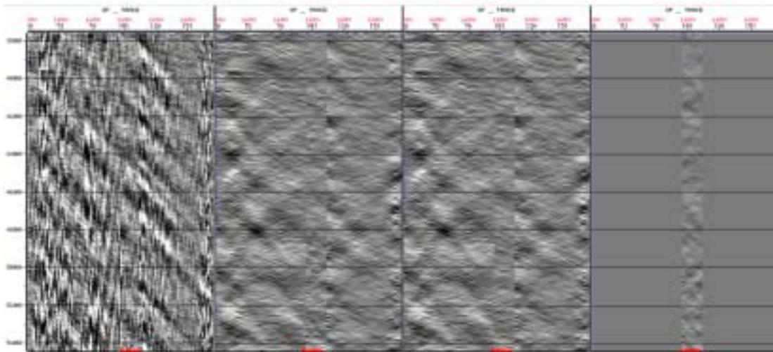
*a.: input                      b.: filter + summing      c.: summing + filter      d.: difference b - c*
