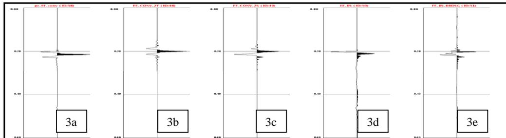
Figure 3 wavelet matching: a: Conventional Far Field (FF) signature with receiver ghost, b) after full zero-phase de-signature, c) after removal of the receiver ghost, d) BroadSeis FF signature, e) BroadSeis after source de-signature only.
