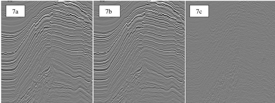
**Figure 7** PSTM stacks for a) conventional and b) BroadSeis after de-ghosting and matching. The difference section c) contains mainly noise.
