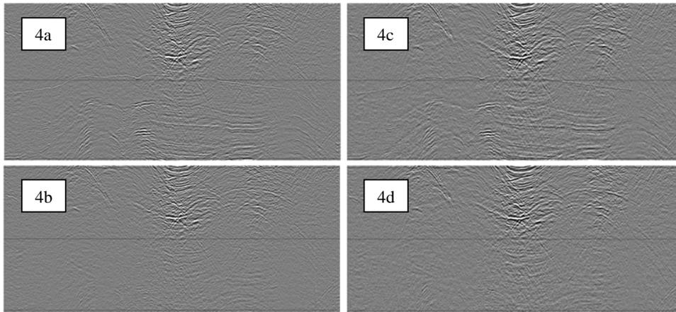
**Figure 4** BroadSeis a) before and b) after SRME. Conventional c) before SRME and d) after SRME.
