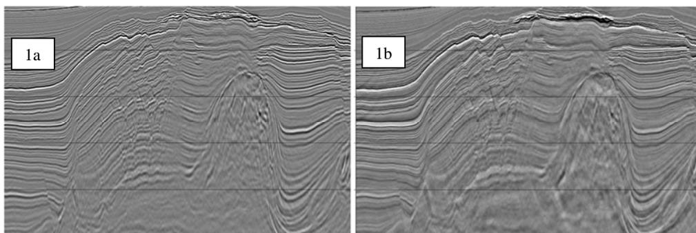
**Figure 1** Crossline PSTM comparison between a) conventional and b) BroadSeis.
