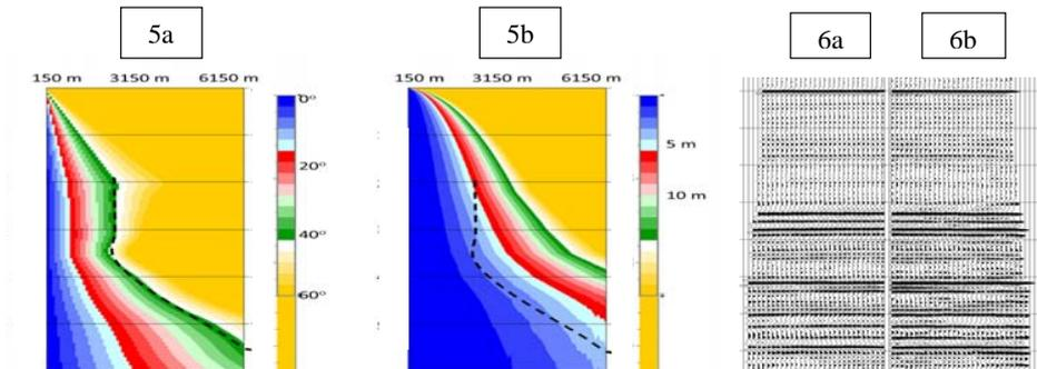
**Figure 5** a) map of incidence angles and b) associated CMP shift due to the variable depth streamer shape.
