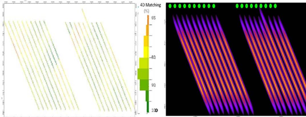
Figure 4. Shot-by-shot 4D-similarity of illumination (left) displayed on survey map and shot-lines flagged with green-acceptable similarity (right)
