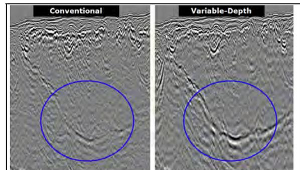
Figure 2: On the left, conventional marine streamer acquisition RTM Saltflood image (20 Hz) over Alaminos Canyon in Gulf of Mexico. On the right, improvement achieved with a variable-depth streamer broadband solution.
