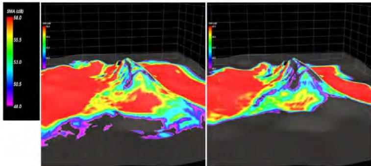
Figure 11: Illumination map with staggered configuration (left) and orthogonal WAZ (right).
