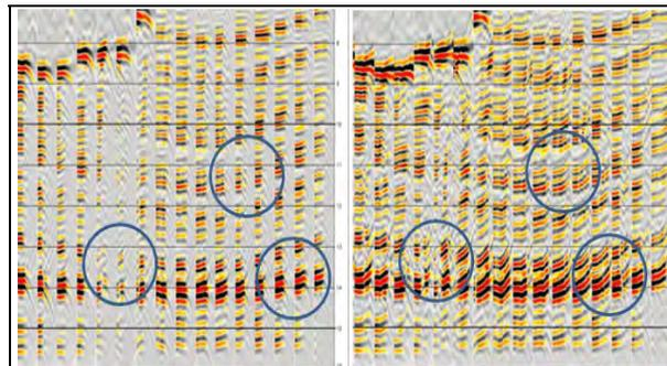
Figure 4: Modeling using SEAM model with a 5% velocity error. The subsalt velocity error is clearly seen on gathers with 16-km offsets (right), while difficult to notice on the gathers with 8-km offsets (left).
