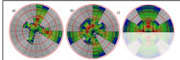
Figure 7: Azimuth and offset distribution for a) North-South lines, b) East-West lines, and c) combination. The red circles represent 5 km, 10 km, 15 km and 20 km offsets. Figure 7c) includes the reciprocity principle. The black rectangle represents what would be covered by a conventional WAZ geometry.
