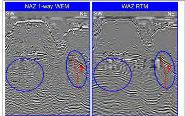
Figure 1: Evolution of subsalt imaging. On the left, a NAZ 2006 dataset and on the right, a WAZ 2009 dataset over the same area. WAZ and RTM significantly improve the quality of imaging. However, some areas are still not well-imaged and require further improvement.
