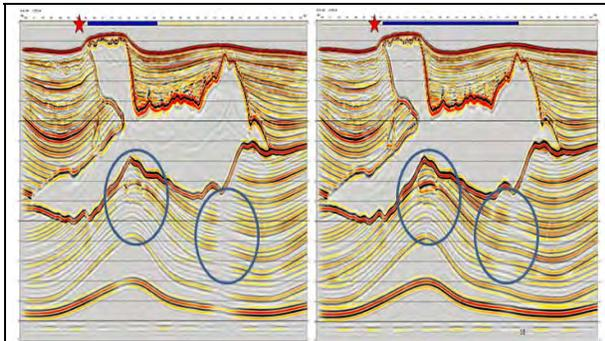
Figure 3: 16-km offsets (right) provide improvement on the imaging compared to the 8km offsets model (left).
