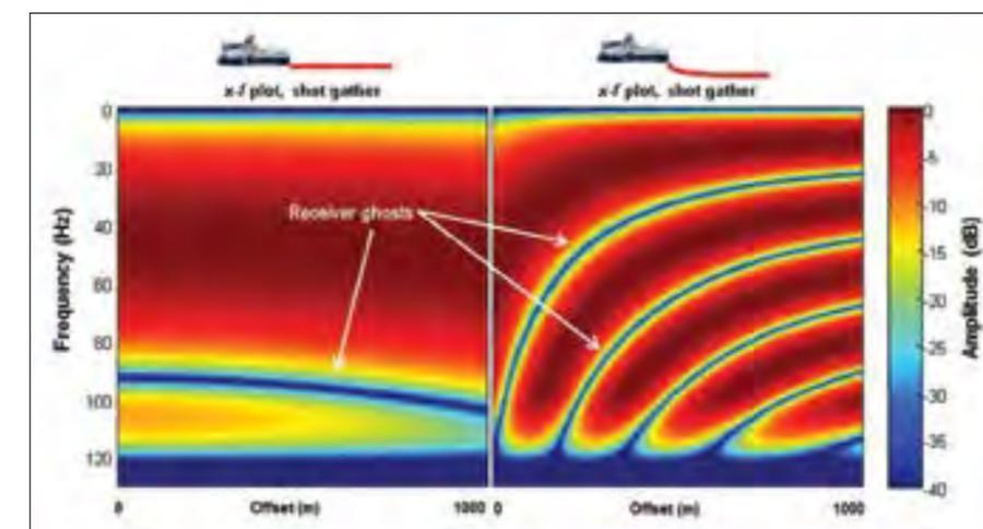
Figure 1. Idealized receiver ghost notch attenuation versus offset for conventional (8-m deep) and variable-depth (6.2- to 36.6-m deep) configurations (before NMO). The improved receiver notch diversity of BroadSeis is visible.
