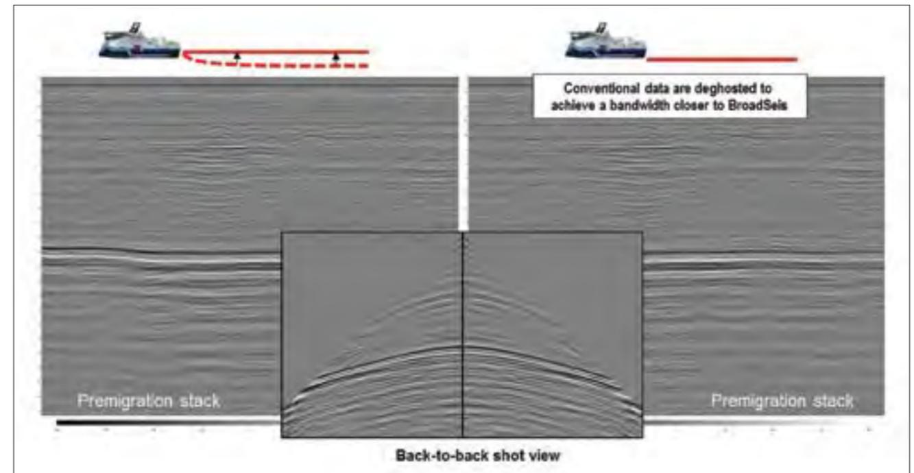
**Figure 7.** Shot gather and stack after codatumming and maximal ghost wavefield elimination applied to both sets of data.
