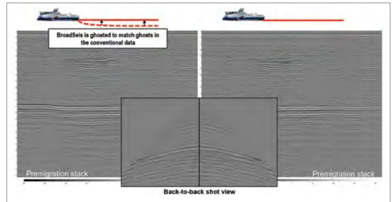
**Figure 5.** Shot gathers and premigration stacks after codatuming of both data sets to a common depth of 9 m.
