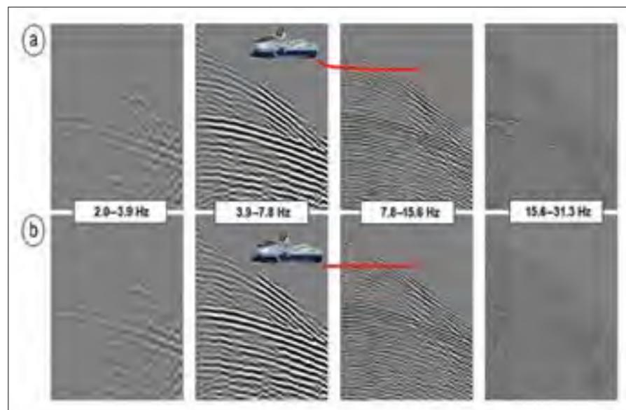
**Figure 3.** Frequency panels of as much as 30 Hz for (a) BroadSeis and (b) conventional tow. Both data sets have undergone denoise processing.
