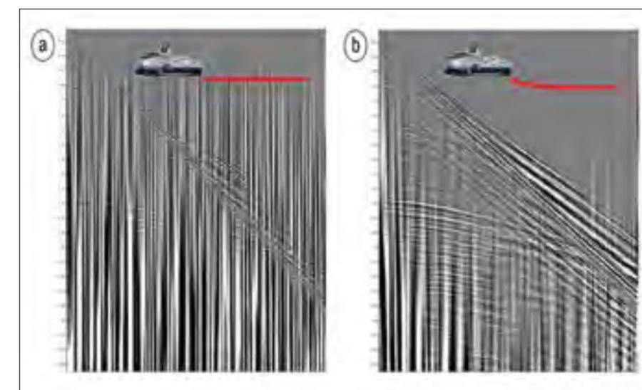
Figure 2. (a) Flat and (b) variable-depth streamer raw shot gathers (shown with  $t^2$  gain).
