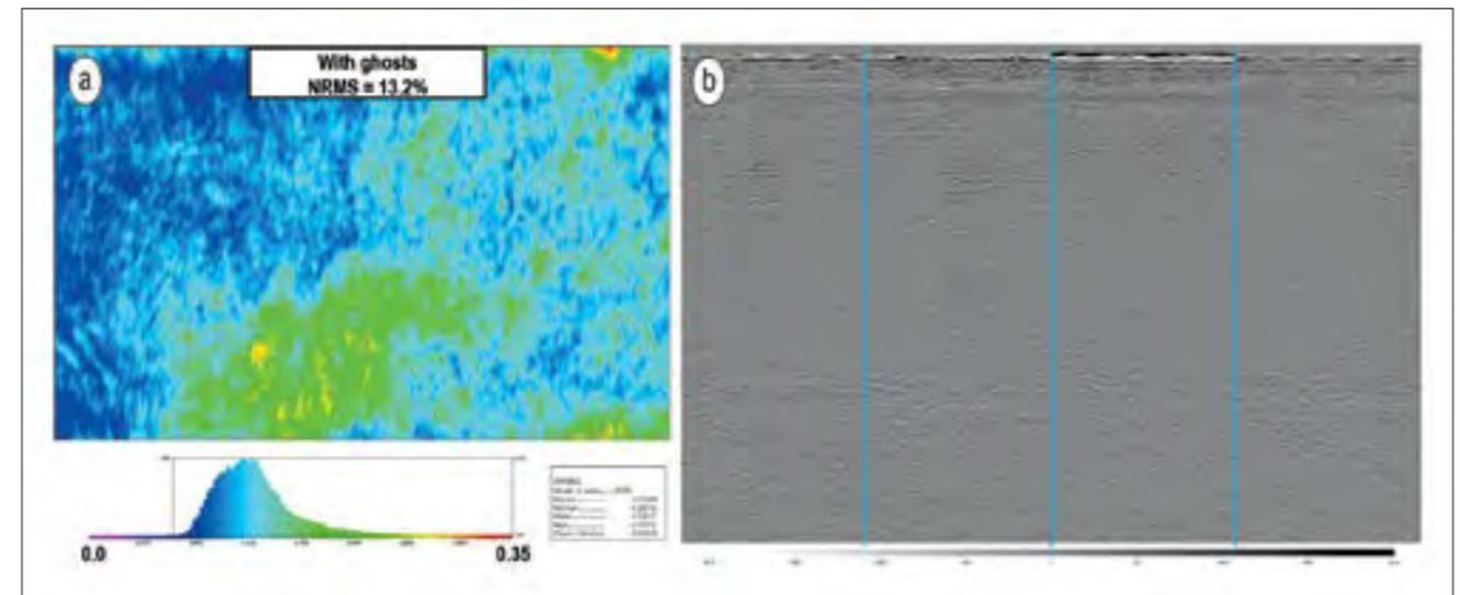
**Figure 6.** (a) Postmigration repeatability analysis of conventional towed and variable-depth streamer data after application of codatumming to a reference datum of 9 m. The BroadSeis data were reghosted at that depth. There is no 4D effect because the two acquisitions were acquired at the same calendar time. (b) The seismic section shows four inlines.
