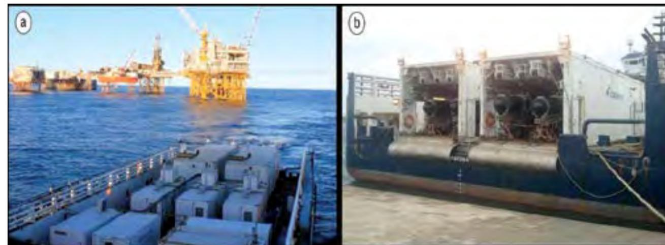
Figure 2. (a) View of the back deck of the supply vessel, presenting the different containers used for seismic acquisition, shown here close to the main Ekofisk platform complex. (b) View of the rear of the vessel, showing both source containers with two subarrays in each.
