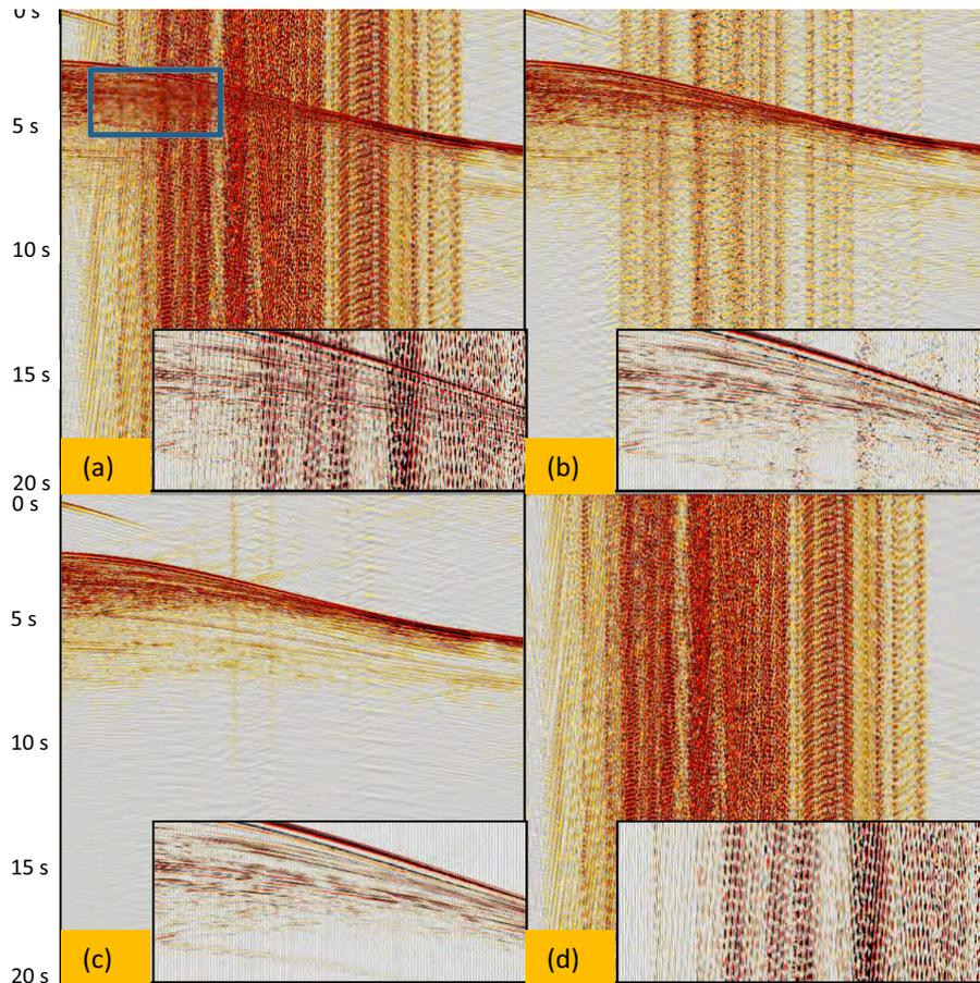
**Figure 2:** (a) A raw shot gather with strong turn noise, (b) the result after low-cut and F-K dip filtering, (c) the result after the coherence-preferred ALTP noise attenuation, (d) the attenuated noise. The subplots are zoomed in displays of a shallow window indicated by the square in (a).
