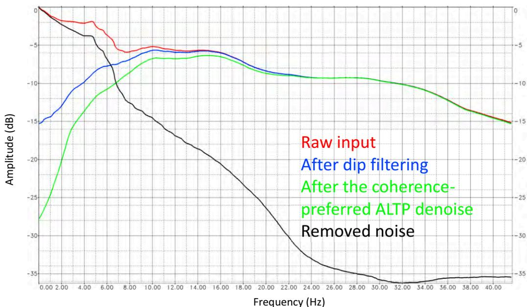
**Figure 3:** The frequency spectrum of the raw input (red), the spectrum after dip filtering (blue) (includes a mild low-cut filter), the spectrum after coherence-preferred ALTP denoise (green), and the spectrum of the removed noise (black).
