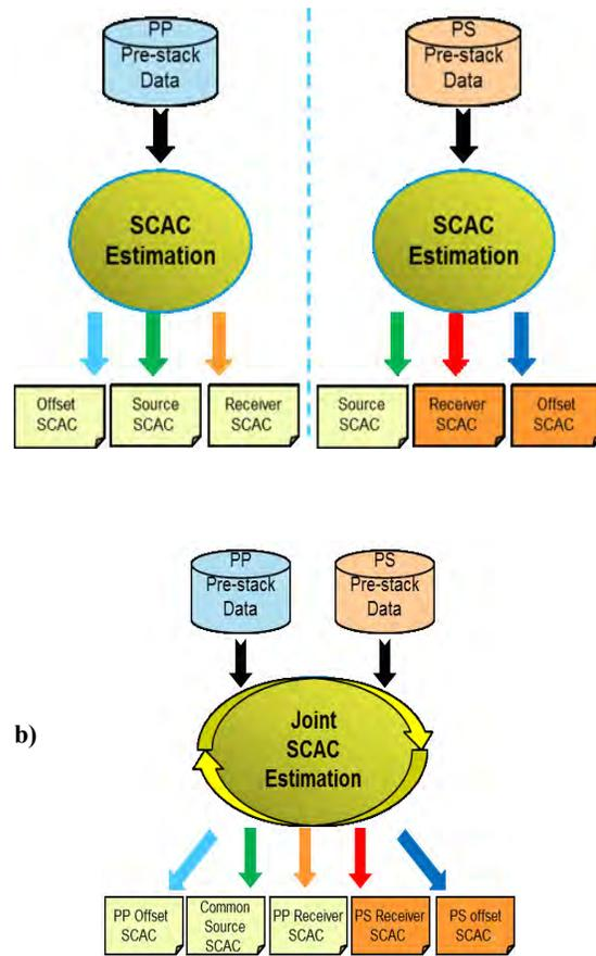
Figure 1: a) description of the conventional parallel SCAC flow; b) description of the simultaneous joint SCAC flow.
