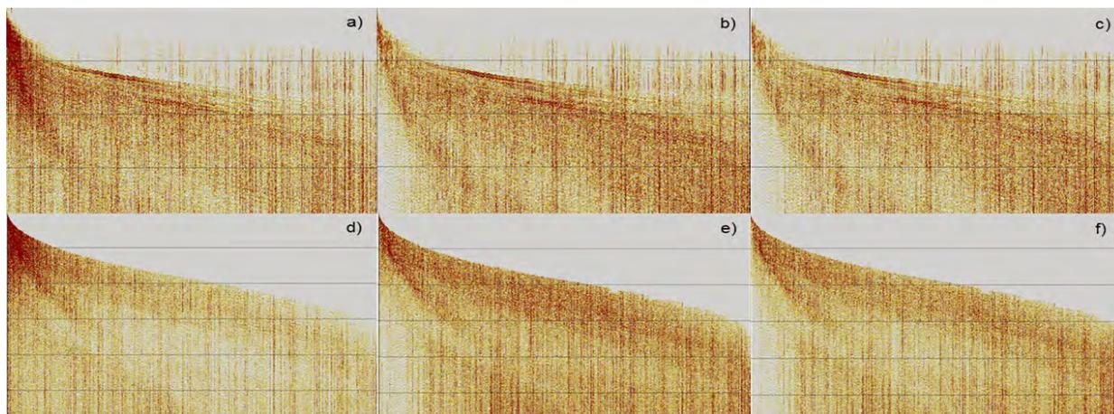
Figure 4: PP receiver gather in PP time, a) Input data, b) After the conventional parallel SCAC flow, c) After the simultaneous joint SCAC flow. - PS receiver gather in PS time, d) Input data, e) After the conventional parallel SCAC flow, f) After the simultaneous joint SCAC flow.
