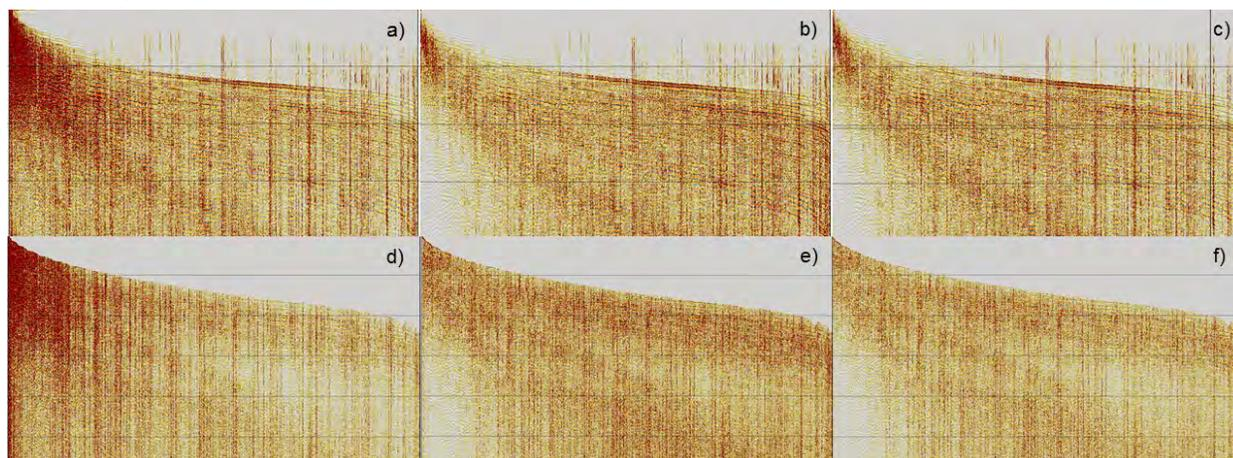
Figure 5: PP shot point gather in PP time, a) Input data, b) After the conventional parallel SCAC flow, c) After the simultaneous joint SCAC flow. - PS shot point gather in PS time, d) Input data, e) After the conventional parallel SCAC flow, f) After the simultaneous joint SCAC flow.
