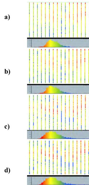
Figure 3: Receiver scalars a) for the PP dataset, computed with conventional parallel SCAC flow; b) for the PP dataset, computed with the simultaneous joint SCAC flow; c) for the PS dataset computed, with the conventional parallel SCAC flow; d) for the PS dataset, computed with the simultaneous joint SCAC flow.
