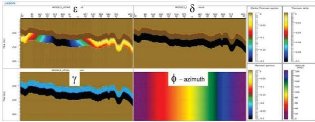
**Figure 3:** The same cross section through the model depicting the three Thomsen parameters and the anisotropy symmetry axis.
