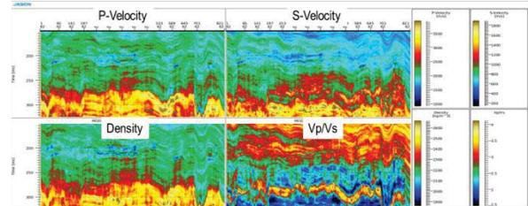
**Figure 2: A cross section through the synthetic model, depicting the isotropic elastic parameters Vp, Vs, Rho and Vp/Vs.**
