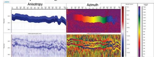
**Figure 7:** The expected  $V_p/V_s$  anisotropy (top) and calculated anisotropy after inversion.
