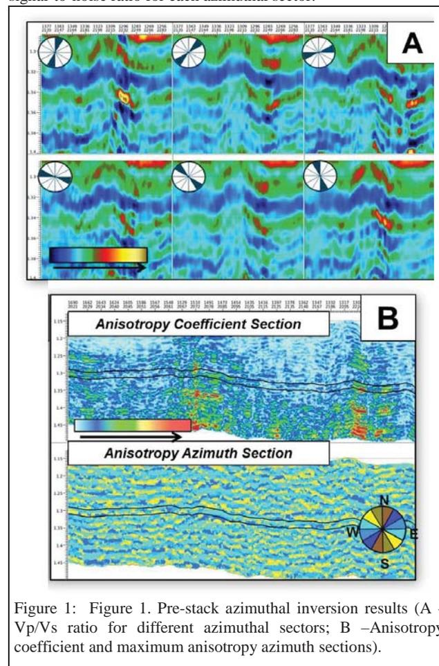
Figure 1: Figure 1. Pre-stack azimuthal inversion results (A -  $V_p/V_s$  ratio for different azimuthal sectors; B - Anisotropy coefficient and maximum anisotropy azimuth sections).
