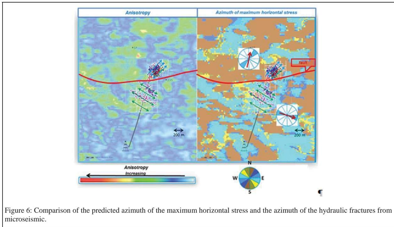
Figure 6: Comparison of the predicted azimuth of the maximum horizontal stress and the azimuth of the hydraulic fractures from microseismic.
