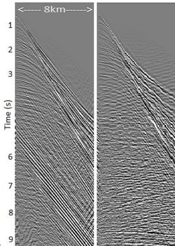
**Figure 1.** Two shot gathers from the North Sea. Left: With SI coming from the front at a distance of ~20km. Right: With SI from the side and tail at a distance of ~70km.
