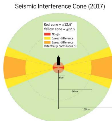
**Figure 3.** A seismic vessel surrounded by its noise cone. This illustration emphasizes the fact that we wanted to avoid having SI coming in broadside.
